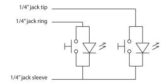
**Mastermind PBC External Switch Wiring Diagram**
