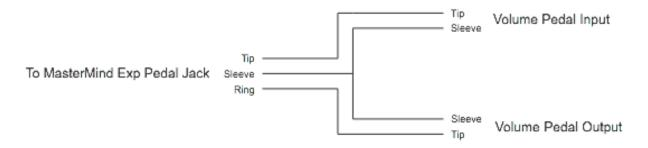
This has the disadvantage that most of the value change will happen at one end of the pedal due to the volume pedal's audio taper. Pedals made specifically to be expression pedals will not have this problem.
